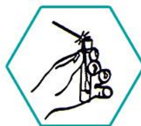
Insert the swab into transport medium and break the handle at breakpoint after sampling.
